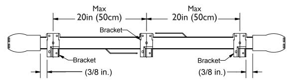
Loosen the screw on the bracket and move the locking arm to the open position. Position the brackets on the track as illustrated below (see diagram below left). Lock the bracket to the track by moving back the locking arm to locking position (see diagram below right) and tighten screw. Note: If your track is spliced, make sure that you place a bracket on the left AND right side of the splice.
