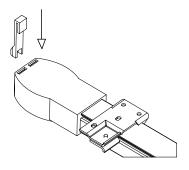
Note: Installers must provide the fasteners appropriate for the conditions at the particular job site. Install brackets onto firm and solid surfaces only. DO NOT install onto dry wall.
