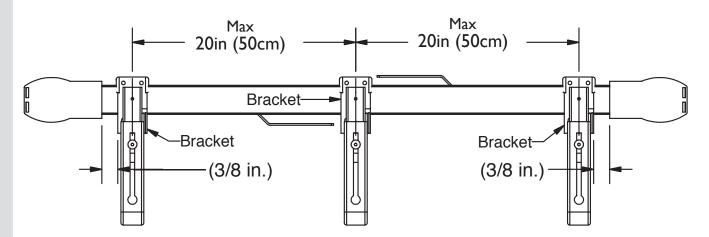
Loosen the screw on the bracket and move the locking arm to the open position. Position the track onto the brackets as illustrated below (see diagram below left), lock the track to the brackets by moving back the locking arm to locking position (see diagram below right) and tighten screw. Note: If your track is spliced, make sure to place a bracket on the left AND right side of the splice.
